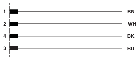
Contact assignment of the M8 plug
